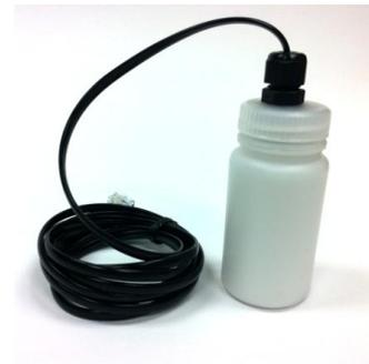
Digital IC Temperature Sensor Configurations: Exposed sensor on the end of a cable (left); Stainless steel sheathed sensors (two sized sheaths) on the end of a cable (middle); Dry granular material filled buffer vial with sensor attached (right)
