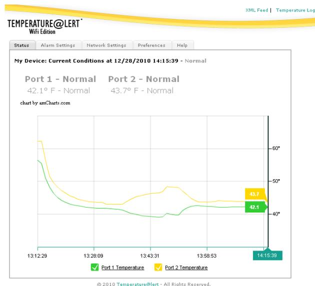
Figure 3: The same Temperature@lert WiFi220 with two temperature sensors after moving them to a household refrigerator compartment.
