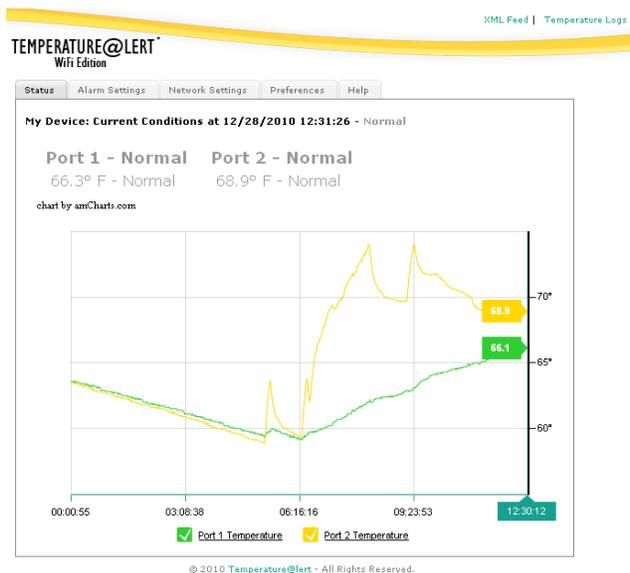
Figure 2: The same Temperature@lert WiFi220 with two temperature sensors showing the effect of a ceiling fan mixing the room air, making floor and eye level temperatures more equal.
