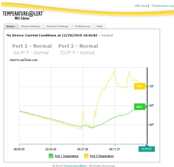
Figure 1: Temperature@lert WiFi220 with two temperature sensors monitoring the floor level (green) and eye level (yellow) in a small bedroom during the night and morning hours.
